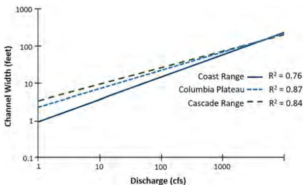
**FIGURE 2** Hydraulic geometry relationships for rivers in different Level III Ecoregions in the Pacific Northwest [Colour figure can be viewed at [wileyonlinelibrary.com](http://wileyonlinelibrary.com)]
